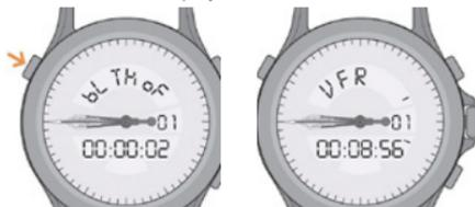
2. A short press of button **A** switches from "VFR" mode to "IFR" mode, and vice versa.
