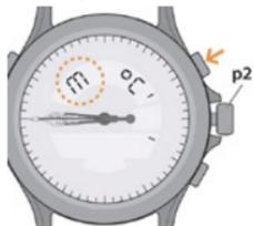
3. A short press of button **B** changes the temperature unit.
