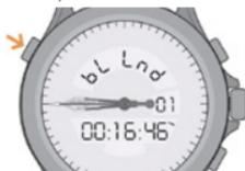
2. A short press of button **B** briefly displays the number of cycles, after which the display returns to "bL Lnd". In the example, the first landing has been made so the number of cycles displayed is 01.
