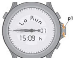
2. A short press of button (A) or (B) allows selection and scrolling in ascending or descending order of the logs of each block, and of the total "to" made up by blocks 01, 02, etc.
