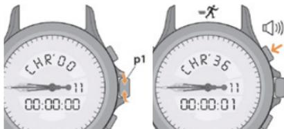
3. A short press of button **A** stops the chrono and the display indicates the result with an "Add" followed by the hundredths of a second and the hours, minutes and seconds underneath. A further press on the button relaunches the timing and adds the time onto the first timing.
