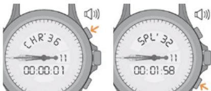
3. A further press on button **B** causes the timing to continue and the elapsed time is caught up with. A third press displays the second split time. The same procedure should be followed for further split times.
