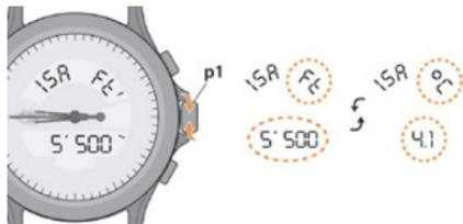
2. A short press of button **A** or **B** allows increasing or decreasing the altitude in steps of 500 feet or 150 meters.
