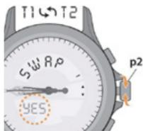
6. Push the crown back to position (p1). Time zones "T1" and "T2" interchange and the hands take the position of the new time "T1".
