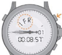
3. A short press of button **B** briefly displays the number of cycles, after which the display returns to "VFR" or "IFR".
